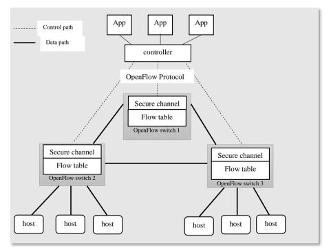
Figure 3. OpenFlow based SDN architecture
