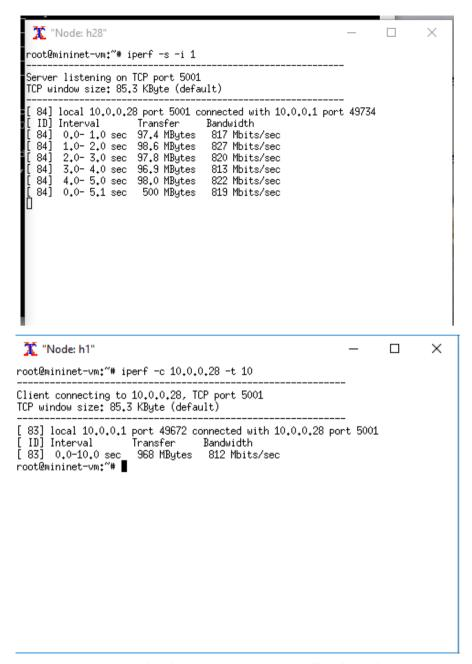
Figure 11. Throughput over TCP connection in Traditional network
