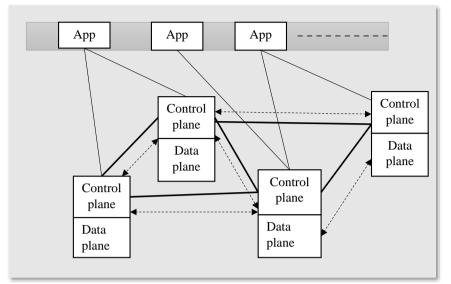
Figure 1. Architecture of Traditional network
