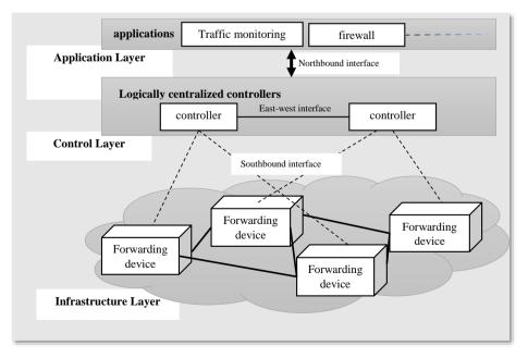
Figure 2. Architecture of SDN
